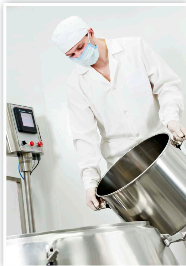
Fig. 1. A blender getting charged with a powder. Note that the bucket discharging the powder should be bonded to the receiving vessel or grounded independently.
