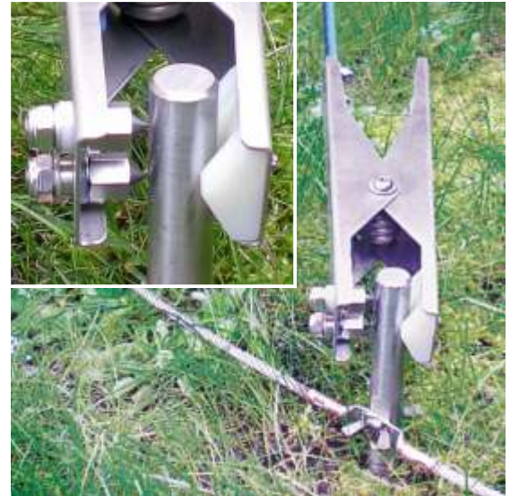
Quick release static grounding clamp supplied with the Earth-Rite MGV attached to buried rod.
