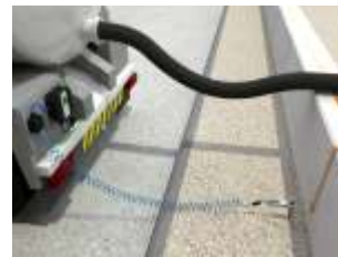
The truck mounted grounding system, the Earth-Rite MGV, tests grounding points to ensure they are capable of grounding trucks.
