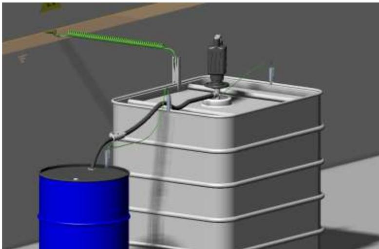
Equipment can only be grounded by ensuring a low resistance connection to verified true earth grounding points (e.g. copper bus-bars). Other equipment used in the process can be bonded to the equipment that is grounded ensuring static electricity does not accumulate on the equipment in the overall system.
